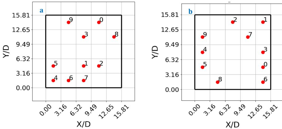
Figure 33: Turbine positioning of initial (a) and optimised layouts (b) for the first MC run
