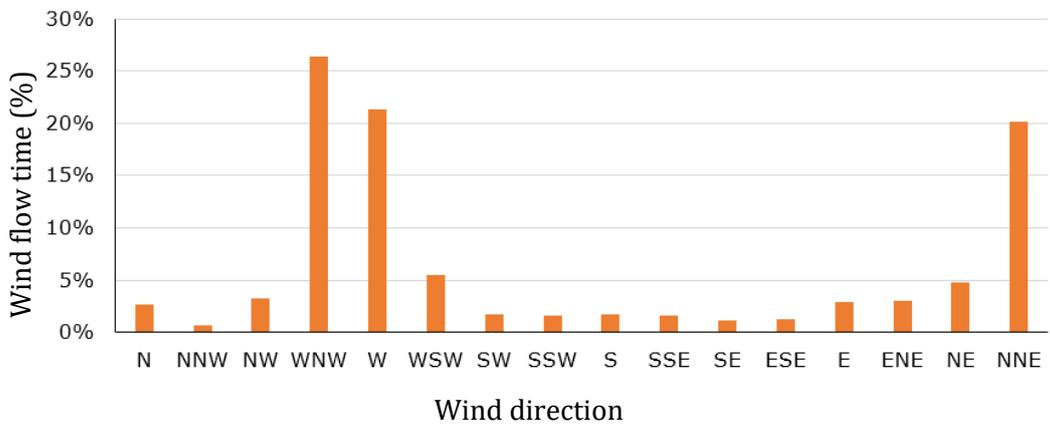
Figure 22: The wind flow distribution in different wind sectors
