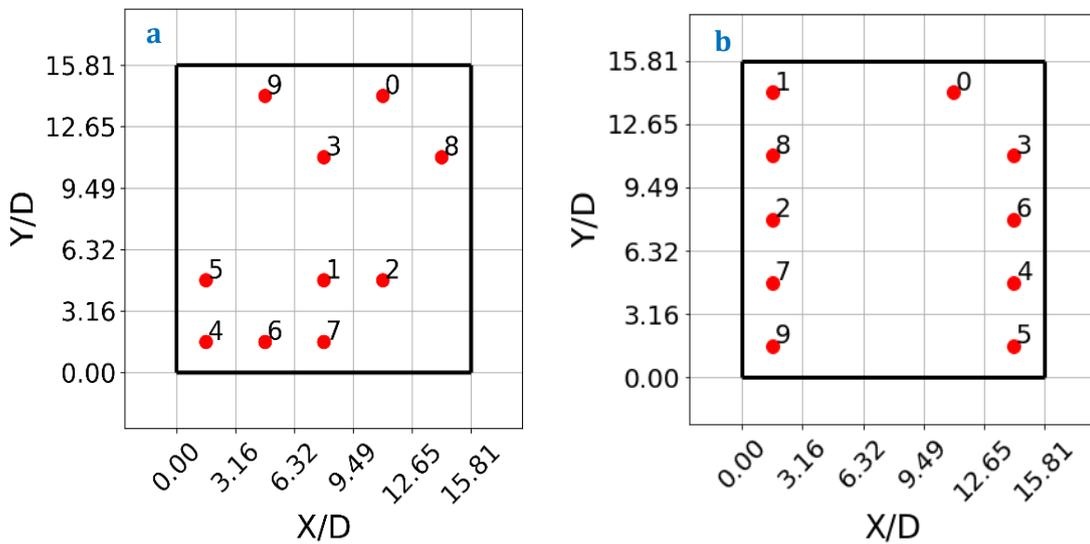
Figure 34: Turbine positioning of the initial (a) and optimised layout (b) for the second MC run
