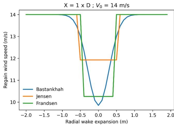
Figure 24: Comparison of different wake models to examine the regain velocity for an inflow wind of 14 m/s
