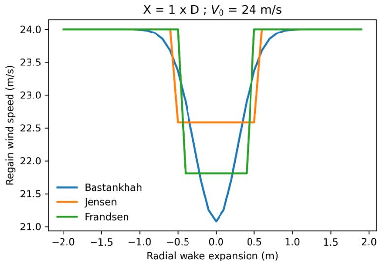
Figure 25: Comparison of different wake models to examine the regain velocity for an inflow wind of 24 m/s
