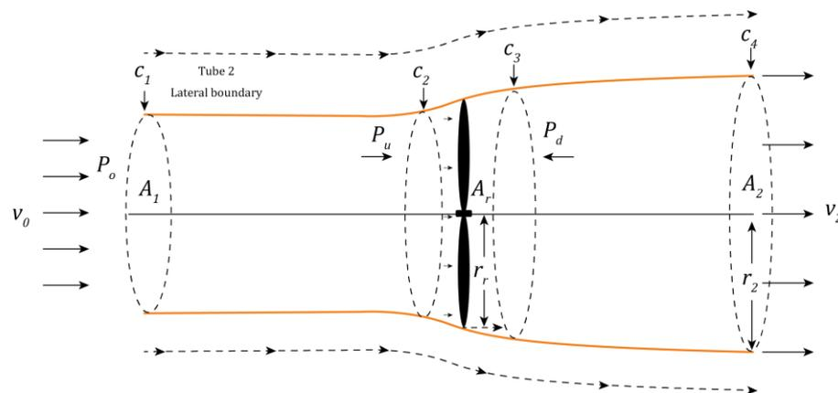
Figure 4: Actuator disk model of the wind stream
