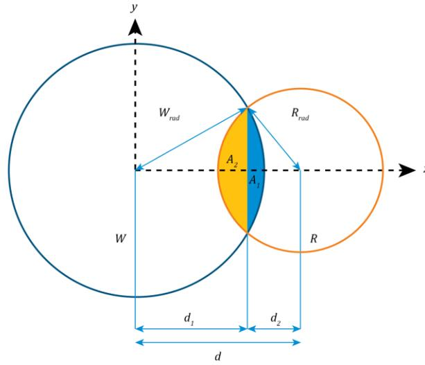
Figure 9: The interaction of wake field and rotor based on the intersection of circles
