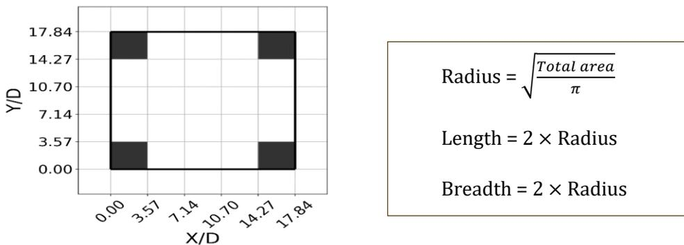
Figure 16: Illustration of the circle layout with an example
