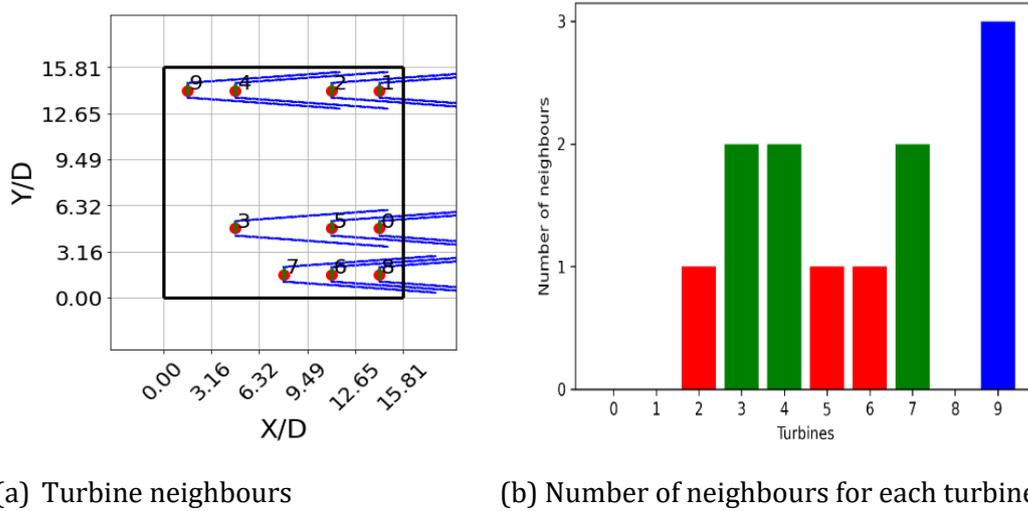
Figure 11: Identified turbine neighbours in the wind farm layout for a wind direction of 270°
