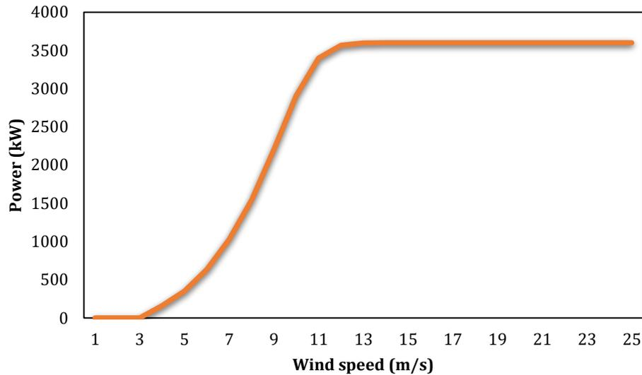
Figure 3: The power curve of a 3.6 MW wind turbine
