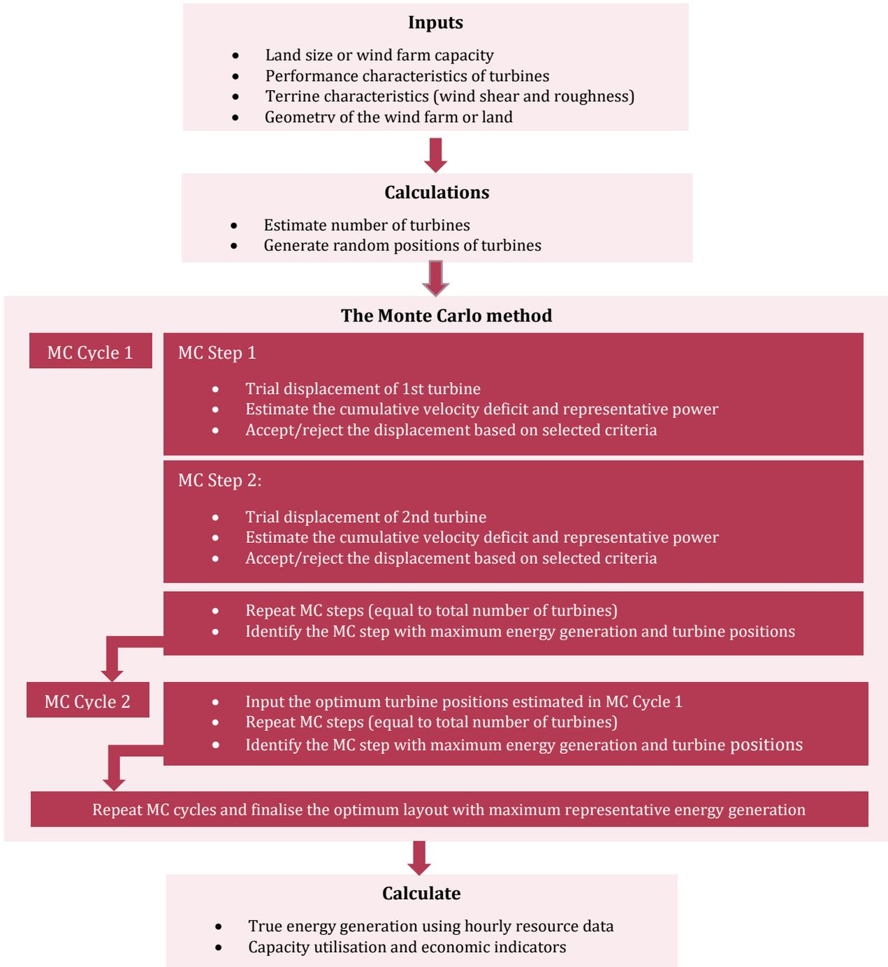
Figure 20: Overall flow chart of the MC simulation
