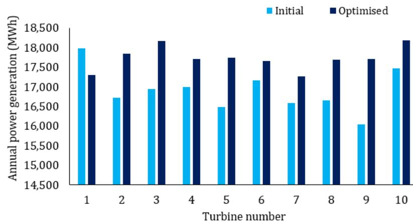
Figure 38: Annual electricity generated by the turbines from the initial and optimised layouts
