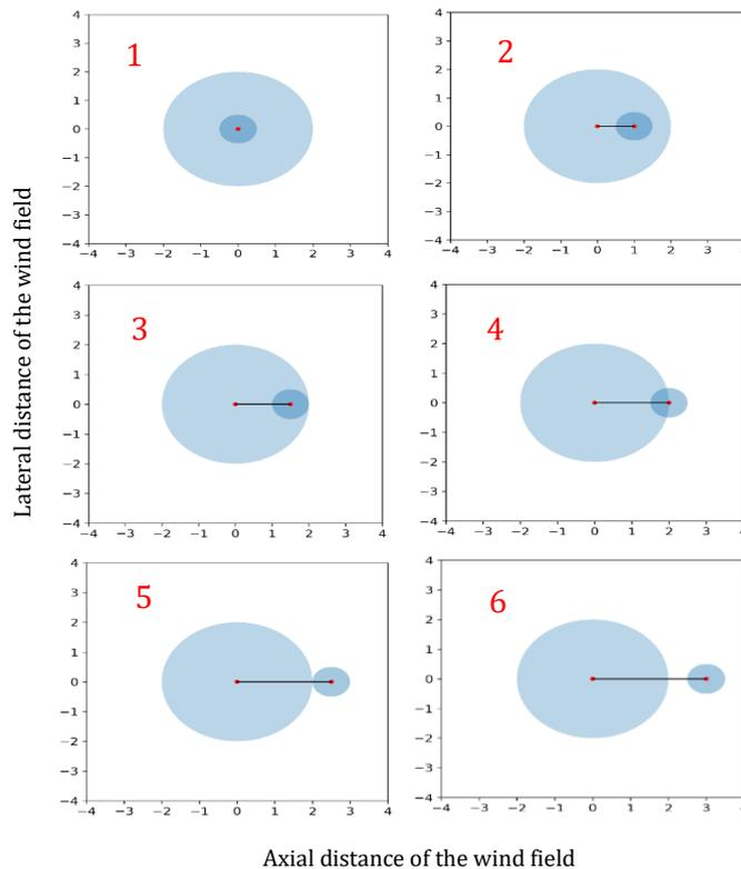
Figure 8: The axial view of various modes of wake field interaction of upstream and downstream turbines
