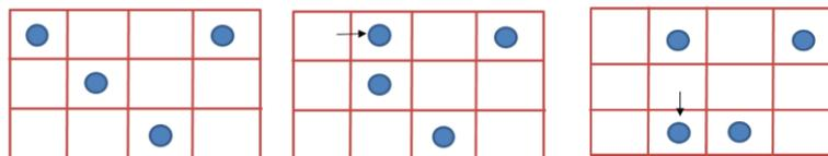
Figure 18: Different MC steps and associated trial displacements
